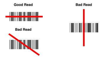
The best focus point for reading most code densities is about 5 inches (12.7 cm) from the unit. To read single or multiple symbols (on a page or on an object), hold the imager at an appropriate distance from the target, pull the trigger, and center the aiming line on the symbol.
